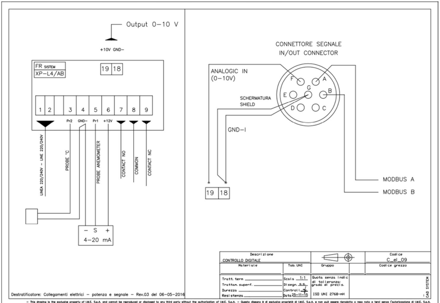
**NB: It is necessary pull the A and B wires down to the control box for the Modbus connection, used for maintenance and diagnostic actions.**
